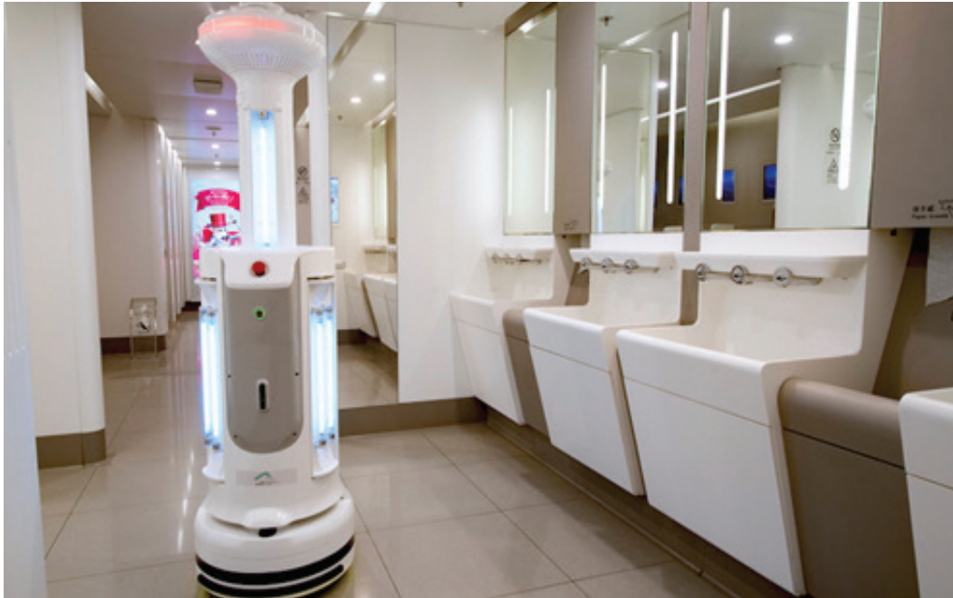
Fig 2. Ultraviolet disinfection robots in Hong Kong airport's restrooms [10].
