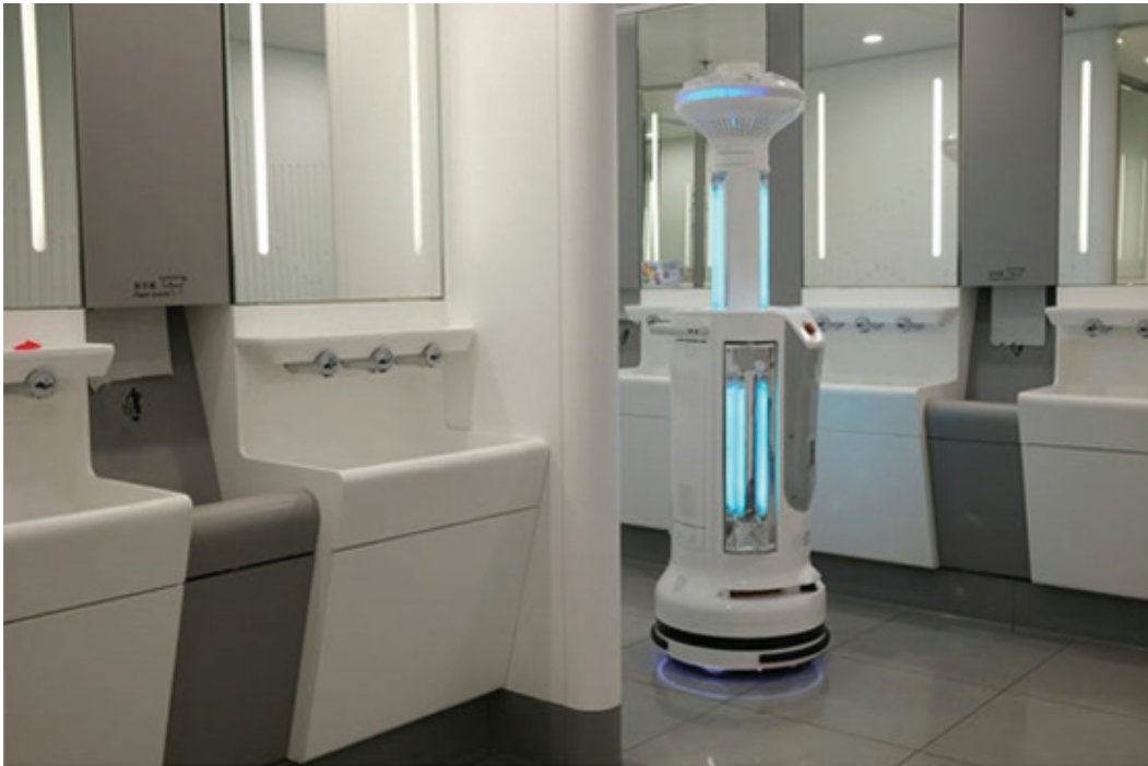
Fig.3. An Intelligent Sterilization Robot (ISR), produced by TMI Rob of China, uses UV light to sanitize, at a toilet, following the coronavirus disease (COVID-19) outbreak, at the Hong Kong International Airport, in Hong Kong, China May 7, 2020. Picture taken May 7, 2020, Tyrone Siu/REUTERS.
