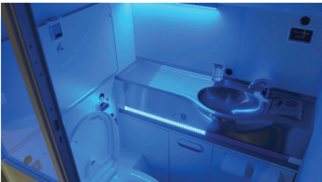
Fig.4. Boeing's self-cleaning lavatory using UV light to kill germs [12].
