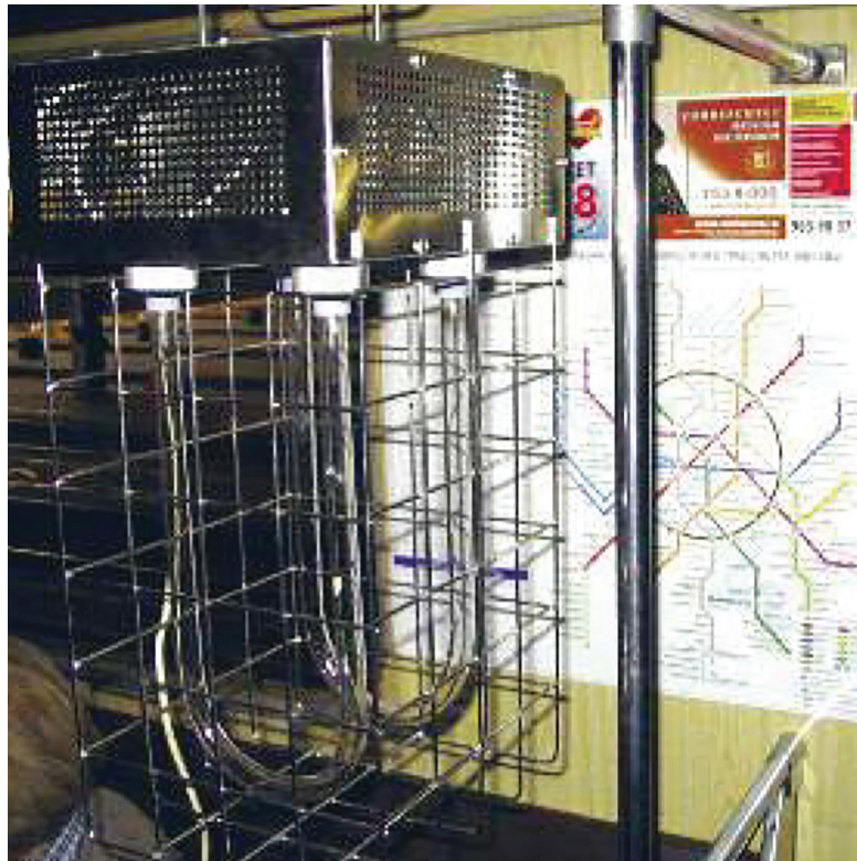
UV system for interior disinfection, with two U-shaped 170 W UV lamps
